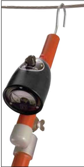
Overhead Voltage-Presence Test can be performed by all models.
