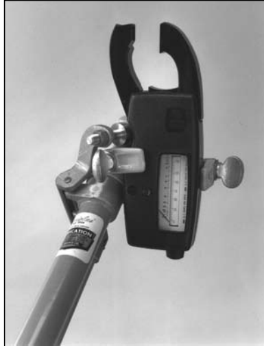
Trigger at end of operating rod controls roller to open and close ammeter jaws.
